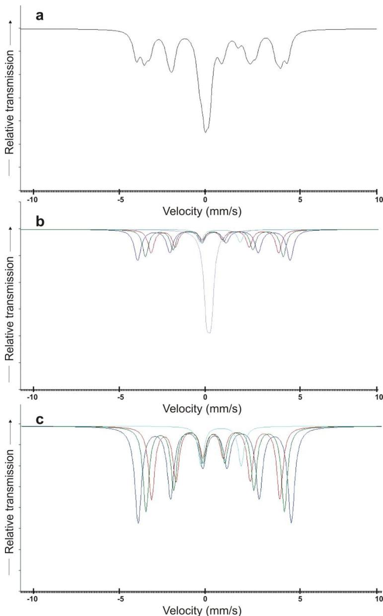
**Fig.5.** Mössbauer spectra of the studied sample. The subspectra colors are the same as in Table 2. A) Mössbauer total spectrum; B) Mössbauer spectrum divided into subspectra; C) Mössbauer spectrum divided into subspectra without magnesio-hornblende subspectrum
